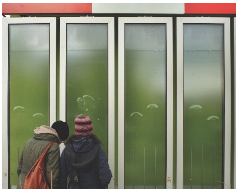
Figure 8A Production of biodiesel from algae. The algae in these containers have the ability to produce a form of oil that can be used as a fuel.
